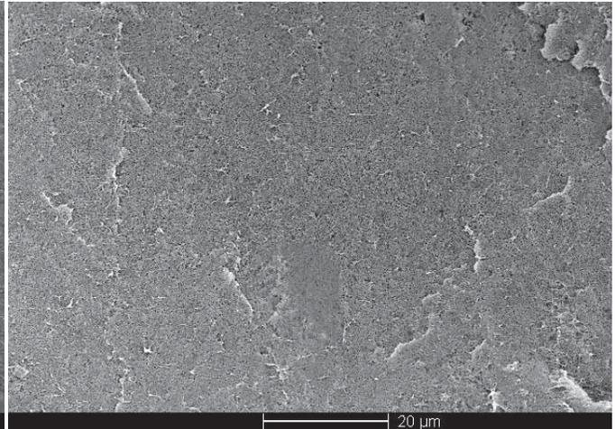
Fracture SEM showing ultrafine pore size of the separator.
