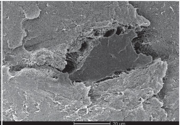
Fracture SEM showing a rubber particle embedded within the separator.
